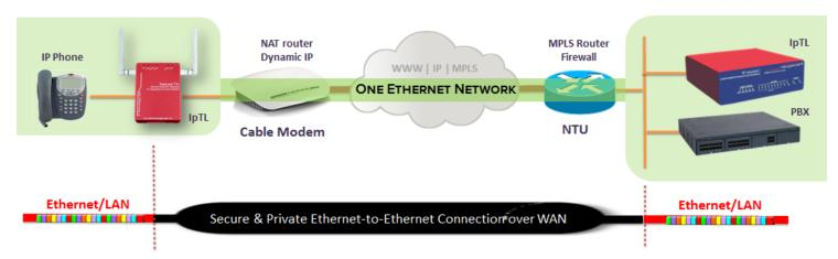
Here you have a remote site with an IP phone connected over a commodity Internet connection. When the secure tunnel is up, the IP phone is able to register to the IP PBX as if it were on the LAN at the headquarters. If the VoIP system uses VLANs for Voice, Video, Data, the IpTL appliance will extend those same VLAN's end-to-end.
