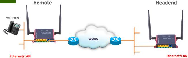
Secure L2 Tunnel – Ethernet Transport
