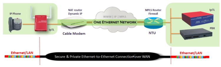
Here you have a remote site with an IP phone connected over a commodity Internet connection. When the secure tunnel is up, the IP phone is able to register to the IP PBX as if it were on the LAN at the headquarters. If the VoIP system uses VLANs for Voice, Video, Data, the IpTL appliance will extend those same VLAN's end-to-end.
